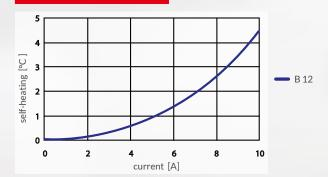
The characteristic curve in the diagram is measured with a thermal switch without any insulation in an oil bath.
